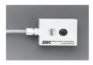
rejecting common false alarms. Continuous self diagnostics perform tests of the detector operation. Each flame detector is tested to respond to a 4-inch diameter isopropyl alcohol (IPA) fire at 10 feet with a 120° field of view.
