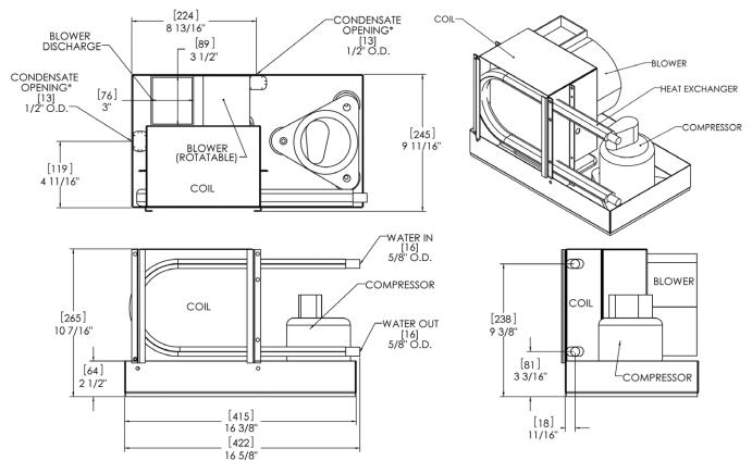
\* ALL CONDENSATE OPENINGS REQUIRE A 5/8" [16] FITTING. ALL DIMENSIONS IN BRACKETS ARE MILLIMETERS. (The control box is always mounted remote from the air conditioner.)
