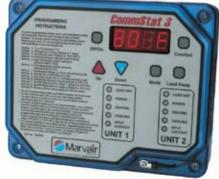
The CommStat 3<sup>™</sup> Controller provides environmental control and the security demanded by the communications industry for a back-up unit. The lead/lag controller insures equal wear on both air conditioners while allowing the lag unit to assist upon demand. The lead/lag changeover is factory set at 7 days, but is programmable in half-day increments from 1/2 to 7 days.
