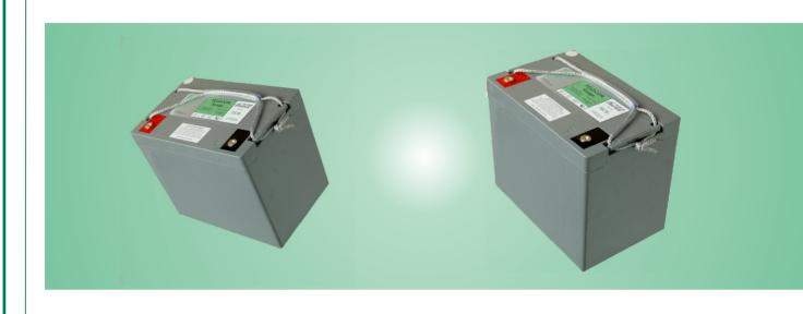
**Model No. TEL 70** (12 Volts, 74.9 Ah at 8 hour Rate to 1.75 vpc) Valve Regulated Lead Acid Battery for communications standby power applications
