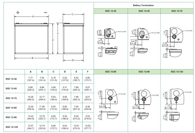
All dimensions in inches and (millimeters). All dimensions are for reference only. Contact a C&D Representative for complete dimension information.
