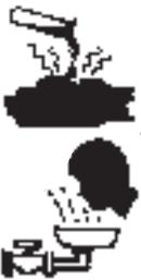
THIS BATTERY CONTAINS **SULFURIC ACID**, WHICH CAN CAUSE SEVERE BURNS. IN CASE OF SKIN CONTACT WITH ELECTROLYTE, REMOVE CONTAMINATED CLOTHING AND FLUSH AFFECTED AREAS THOROUGHLY WITH WATER. IF EYE CONTACT HAS OCCURRED, FLUSH FOR A MINIMUM OF 15 MINUTES WITH LARGE AMOUNTS OF RUNNING WATER AND SEEK IMMEDIATE MEDICAL ATTENTION.
